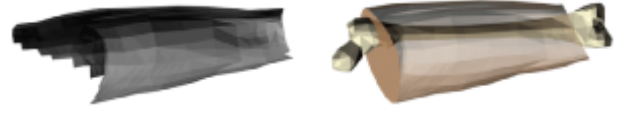
Figure 2: Modeling of a thigh finite element model using a skeleton and CSG operations.
